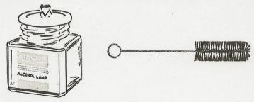
To clean your test tubes after each experiment use your test tube brush.
